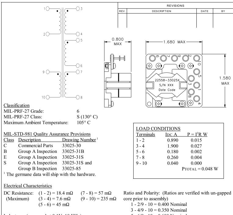
Inductance (measured at 0.1V, 10 KHz): Lo  $(3 - 4) = 34.3 \mu H \pm 10\%$  IDC = 0
