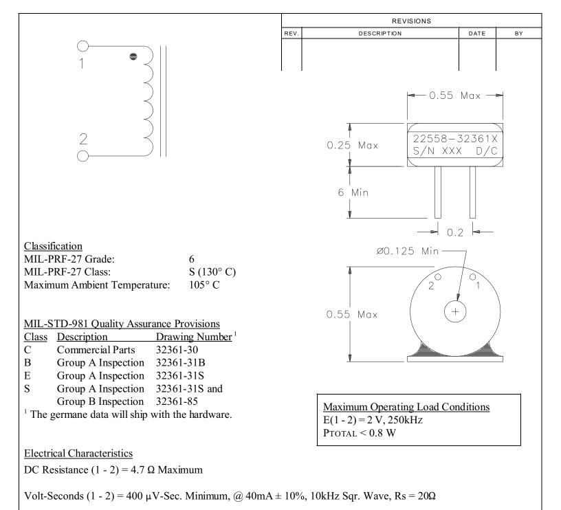
Ratio and Polarity  $(3 - 4/1 - 2) = 0.00400 \pm 0.00003$  (Note: 3 - 4 is 1 turn test winding with the Start on the Lead side of the Transformer)
